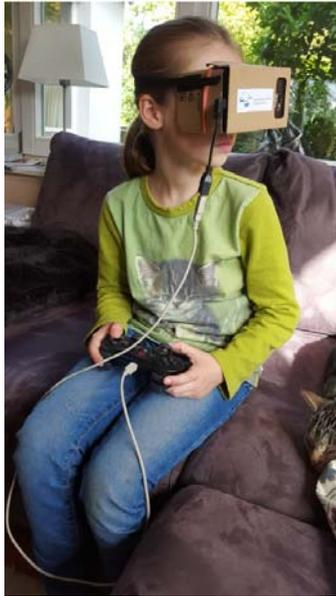
**Figure 2:** Playtesting a VR experience with (wired) game controller in a first explorative usability test on a modified google cardboard. The cardboard is currently the lightest VR solution. Both hands are required for interaction.
