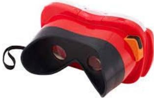
**Figure 1:** The View-Master (Mattel) is the only HMD designed for children. It is compatible with Google Cardboard VR platform. This HMD has a solid hardware, but lacks IPD adjustment. It has to be held by users with at least one hand.
